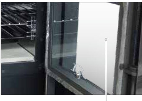
Oven door with double glazed window and a thermometer
